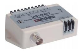
The Vigitron Vi6100DT is an advanced active device that transmits color or B&W video and data over separate point-to-point unshielded twisted pair wires at distances up to 6000 feet (1830 m). The Vi6100DT uses Category 2-7 twisted pair wires, is easy to install and cost effective. It is designed to be paired with Vigitron Vi6100DR active video and data receiver.
