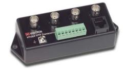
The Vigitron Vi1004 is a passive transceiver hub that transmits video over unshielded twisted pair (UTP) wires, point-to-point, for distances up to 1000 feet (305 m)\*. It is used with Vigitron passive transceivers such as VB1001 to support "up-the-coax" PTZ signals. This Hub use Category 2-5 twisted pair wires, is easy to install, cost effective, and do not require power.
