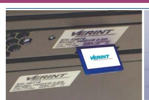
An externally accessible SD flash card for DVR properties facilitates service and future application integration.
