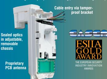
At the heart of the *Mirage* lies an advanced microprocessor. **Neural based environment learning** provides the detector with real intelligence, enabling the PIR circuitry to continually monitor the installation, adjusting detection criteria to ensure optimum catch performance while maintaining maximum false alarm immunity.
