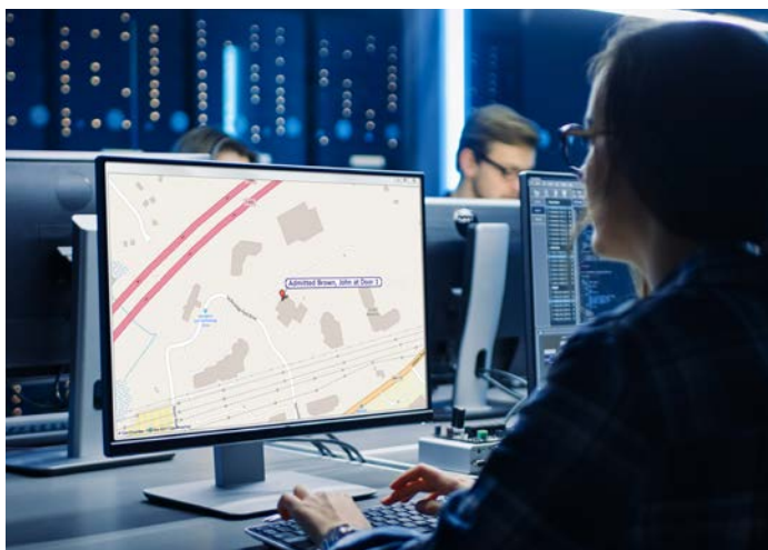
C•CURE 9000 monitoring screen showing GIS location of C•CURE Go Reader card swipe activity
