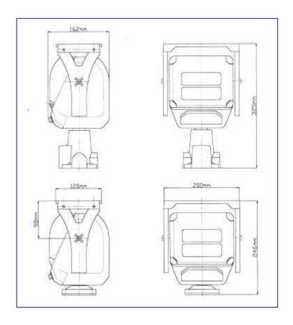
The Shawley Earl PT 565 head is the leader in the range of quality built, versatile and precision designed pan and tilt units, with proven reliability in town centre and traffic monitoring applications. The Earl is the first choice for performance, flexibility and serviceability. Ruggedly constructed in a die cast aluminium case the Earl provides a compact but powerful unit with a load capacity belying its size.
