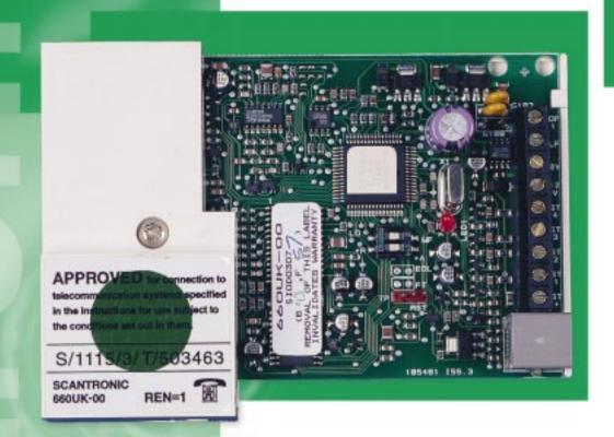
The 660 is a wire-in auto dialling speech/digital communicator unit, designed to be discreetly fitted in a Scantronic, or any other manufacturer's alarm control panel.
