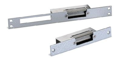
**Electric strikes** provide remote release of a locked door. They allow the door to be opened without retracting the latchbolt. This occurs by the release of the electric strike lip (sometimes called a keeper or gate). When the door closes the beveled latchbolt rides over the lip and falls into the strike pocket. A door can be set either as Fail Safe (loss of electrical power opens the door) or Fail Secure (loss of electrical power locks the door).
