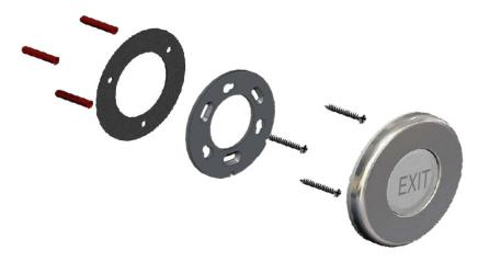
Fix the backplate to the wall with the stainless steel screws provided in the fitting kit. The small slot in the plate edge should be positioned at the bottom.
