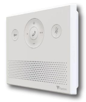
Entry is a door entry system that works standalone or alongside Paxton's Net2 access control, combining door entry with key features of Net2. Entry consists of 3 components that auto-detect on set up; external panel, interior monitor and door control unit. Entry is a plug and play solution that comes with a range of panel options and is suitable for a wide variety of sites.
