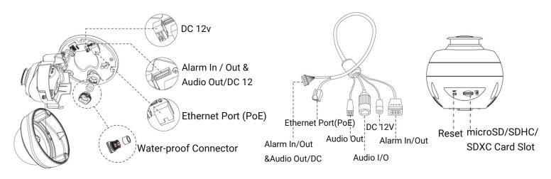
Note: The cable is connected with the interface board by default.
