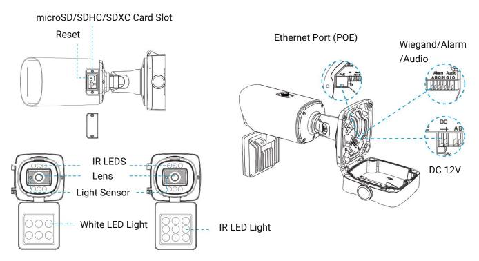
Note: Switching to web side to use Wiegand and Alarm Output.
