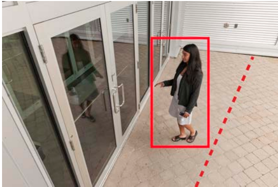
The "Tripwire" analytic triggers an alarm when a person crosses the defined line.
