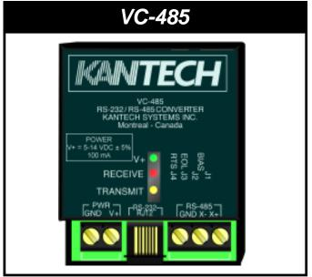
The **VC-485** is an RS-232 / RS-485 protocol converter primarily used to connect a PC to a KT-200/KT-300 controller. The maximum bus length is 5 km (18,000 feet, when line repeater is used) and 1,2 km (4,000 feet) for EntraPass & WinPass when using Ethernet Grade 3, unshielded, two twisted pair cable (Belden # 1227A recommended). Two VC-485's may be connected back-to-back to be used as a line repeater in order to extend the RS-485 communication bus.
