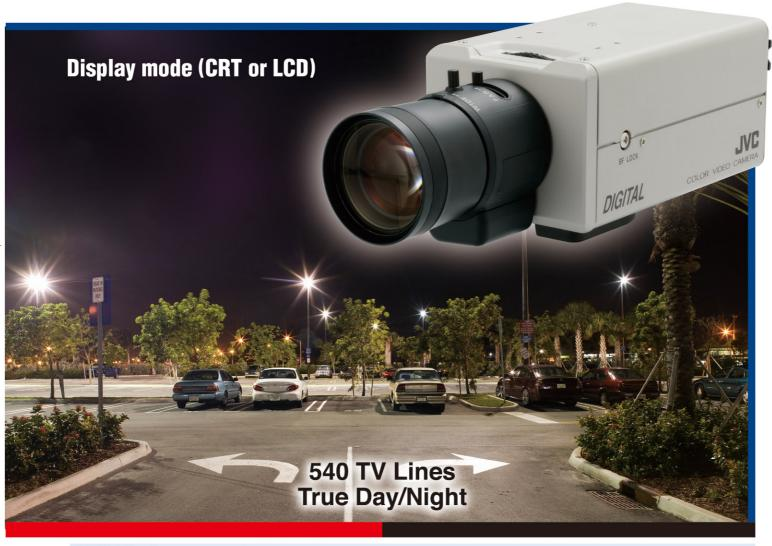
IR ON/OFF function The camera's IR cut filter switches itself automatically on or off according to whether it is day or night. Thus one single camera can be used for unattended 24 hr operation, providing colour images by day and B&W by night.
