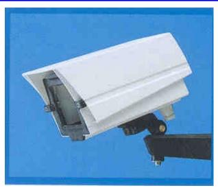
Innovative weatherproof housing for indoor/outdoor installations of ICD-501, Super Cube DVSP Color Camera. Made of specially mixed NYLON, it is small, good-looking, strong and light as well. Thanks to the specially designed sunshield, integrated with the housing to allow air circulation, this model may be ideal to be installed in every environment including tropical ones.
