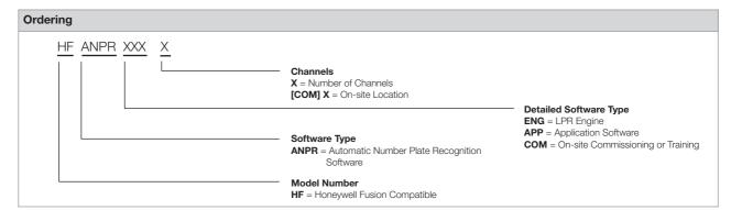
**NOTE:** To utilise Fusion ANPR software, HF3LICDATA and HF3HWUPGCPU must also be purchased separately. **NOTE:** Honeywell reserves the right, without notification, to make changes in product design or specifications.
