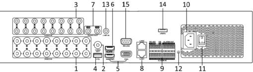
**NOTE** The rear panel of DS-8108/8116HUHI-K8 provides 8 video input interfaces.
