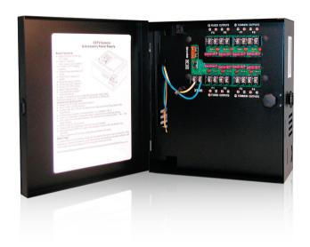
The PWR-24AC-8-7 is a CCTV power center engineered to manage remote camera and accessory power requirements. The PWR-24AC-8-7 distribution module is designed with 8 individually fused outputs for powering up to 8 CCTV cameras and accessories. It will provide 24 Volts AC via distribution to eight fused outputs with a total of 7.25 Amps continuous supply current. The PWR-24AC-8-7 power center is housed in a premium lockable heavy gauge metal enclosure.
