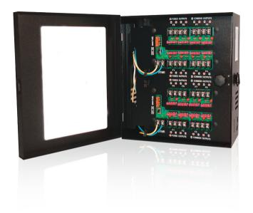
The PWR-24AC-16-14 is a CCTV power center engineered to manage/remote camera and accessory power requirements. The PWR-24AC-16-14 distribution module is designed with 16 individually fused outputs for powering up to 16 CCTV cameras and accessories. It will provide 24 Volts AC via distribution to sixteen fused outputs with a total of 14.5 Amps continuous supply current. The PWR-24AC-16-14 power center is housed in a premium lockable heavy gauge metal enclosure.
