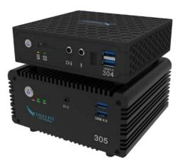
The Eagle Eye Bridge acts as a gateway from your premises to the Eagle Eye Cloud Data Center where your video is stored and managed by the Eagle Eye Cloud VMS. It provides video buffering, a secure connection, bandwidth management, and monitoring of cameras.
