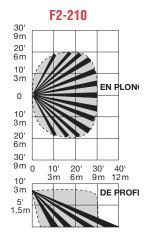
30 x 40ft (9 x 12m) Coverage (max.Lx max.W) : MW range adjust
