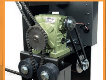
Full Size Gearbox heavy-duty 30:1 ratio gearbox
