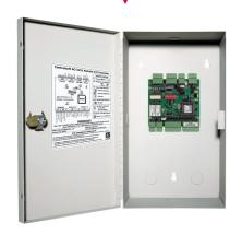
**AC-4311** I/O controllers extend the digital inputs and outputs available on system controllers. Each AC-4311 controller provides eight digital inputs and eight relay outputs.
