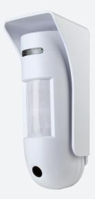
VST-892EX-HD-BUS is a hardwired Outdoor HD PIR Motion Sensor Camera, which is capable of sending wired signals and capturing high definition images (picture quality of up to 1280 x 720 pixels) to the Control Panel upon movement detection via the wired BUS system. VST-892EX-HD-BUS is capable of leveraging alarm image transmission speed, with QVGA in less than 4 seconds, and VGA in just 12 seconds, making visual alarm verification efficient and real-time.
