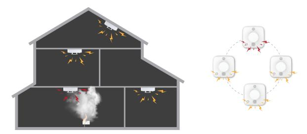
Serial connection enables all connected smoke alarms to sound together when one of them is triggered
