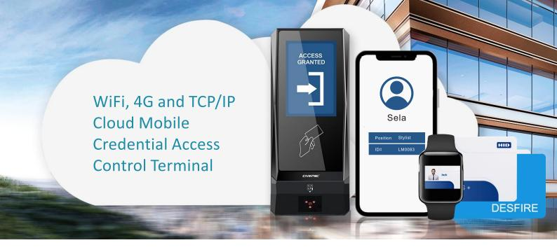
CT9 family is Linux based HTTP/HTTPs server centralized terminal with wireless 4G, WiFi and TCP/IP Ethernet suitable for both LAN and Internet cloud server software communication. It supports both of online server real-time monitor HOST mode and standalone access control Local mode, perfect for multiple IoT & access control solutions. With IP65 ratings, CT9 family is weather resistant to rain, dust, strong sunlight, ideal for various rugged environments installations.
