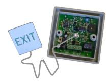
Plate can be fixed remotely from electronics
