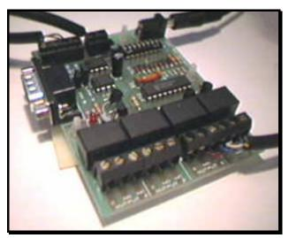
The SOM1 is equipped with an address switch which allows for up to 256 modules to be connected to a single PC Serial Port thus allowing a maximum of 1024 relays.
