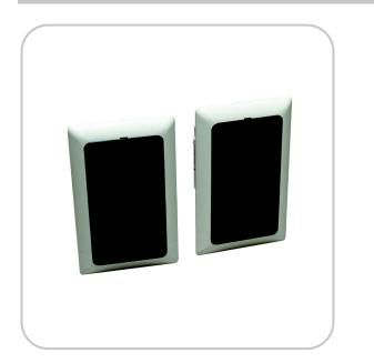
The DS433i is a single-beam, indoor, flush mount photoelectric detector that is designed to mount in a standard single gang box. Its flush mount enclosure makes it an ideal choice where aesthetics are a concern. Internally pointable optics and the ability to mount in a standard single gang electrical box make it easy to install, especially for pre-wired applications.
