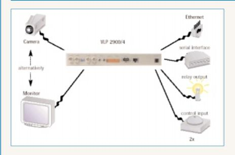
VLP 2900 delivers unidirectional, live video monitoring of remote sites, events and people. The device enables the transmission of video pictures from up to four connected cameras via existing computer networks over any distance.
