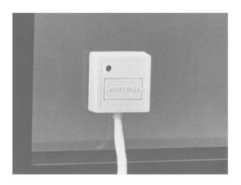
The Aritech GS 110 glassbreak detector has been designed using the latest electronic techniques. This enables the detector to contain all the necessary circuitry for excellent detection whilst filtering out and rejecting all unwanted signals that would normally result in a nuisance alarm(s), e.g. ultra-sound, radio frequency interference, etc.
