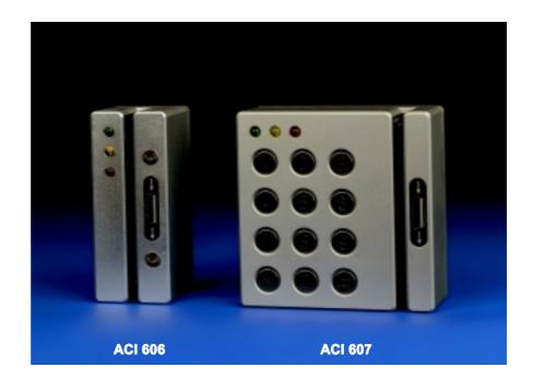
The reader can be mounted beside the door to be controlled. Anyone requesting access must swipe a magnetically encoded card through the slot on the reader. The reader is connected to an Aritech controller which contains the electronics to release the door. The reader can also be equipped with a keypad.
