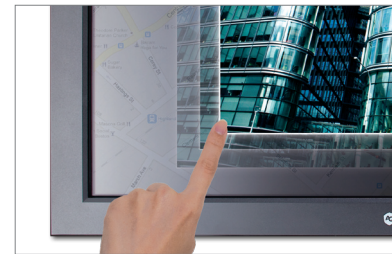
Advanced optical touch technology for accurate, zero-pressure response multi-touch gestures* *Compatible for only dual-touch gestures
